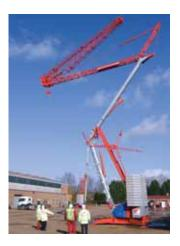
Kier Plant has added a contingent of self-erecting remote controlled cranes to its growing fleet. The Potain Igo 50s have a maximum jib length of 40 metres and can lift up to four tonnes. These electrically-operated cranes are clean and quiet to run and are used mainly or small, low-rise residential and brownfield sites where space in restricted.
